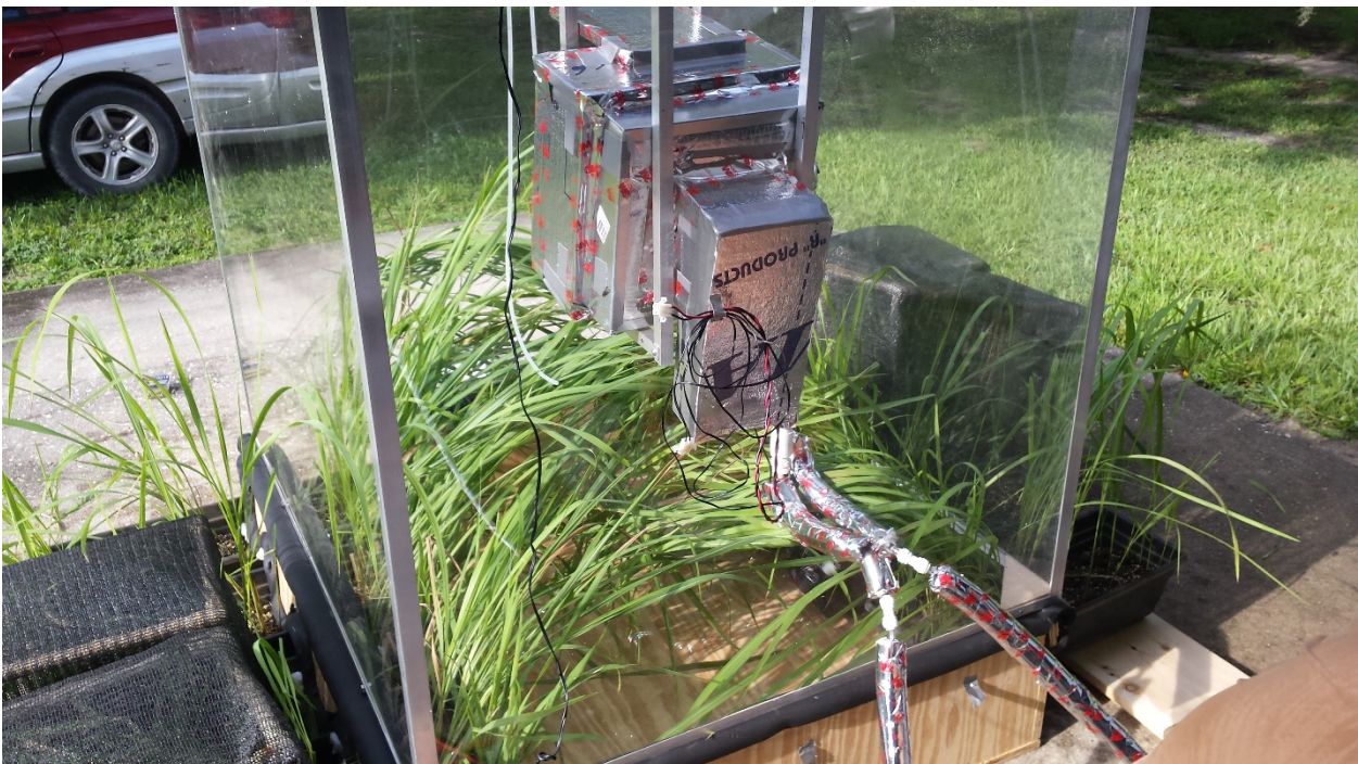
Image 2: Chamber installation with environmental controls (temperature, relative humidity)
