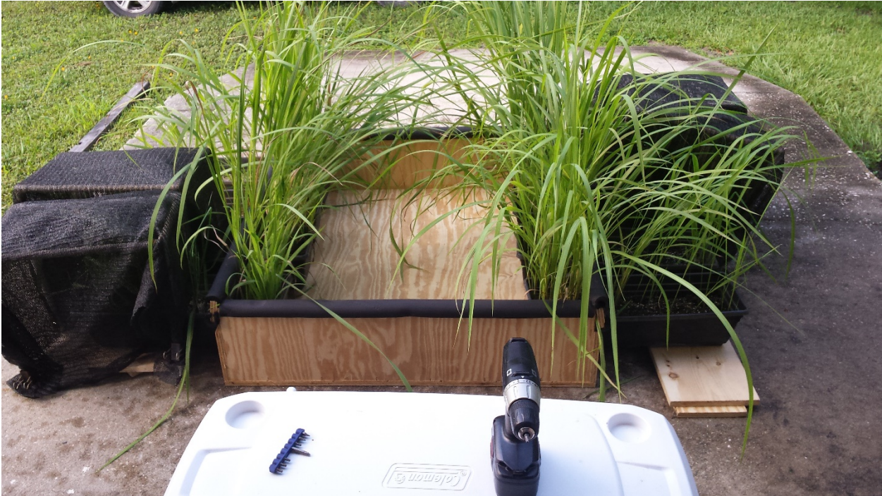
Image 1: Chamber base design isolating parent ramets (inside chamber) and daughter ramets (outside)
