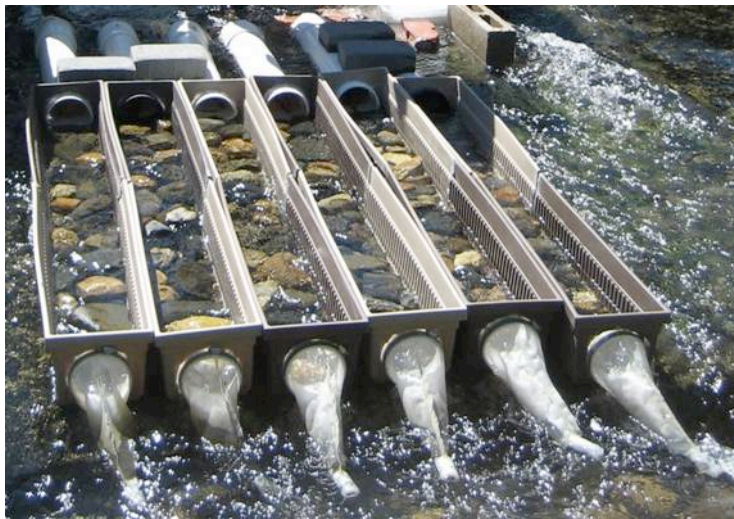
Figure A1. The experimental channels used in the density, excess food, and canopy experiments. The photograph is of day 6, block 1 of the excess food experiment. The PVC pipes at the front of each channel contain the upstream driftnets.
